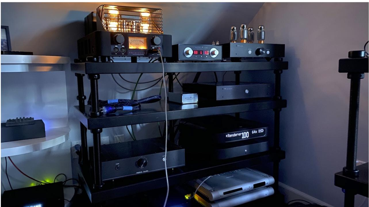
**3. The Setup.** The signal chain is NAS—>Cisco Switch via fiber—>Roon Nucleus+—>MSB Select II w/ Network Renderer 2—>Trafomatic Primavera. ICs are Iconoclast. Power cords are Cerious Graphene. The MSB has a Gigafoil 4 and .5m BJC Cat 6 Ethernet in front of it. The Nucleus+, GigaFoil, and Cisco are powered by a Keces P8 [I share this for info only, not to start a cable/power supply/network discussion].
